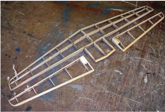
Nothing complicated here—the horizontal stabilizer and elevators are built-up balsa structures.
