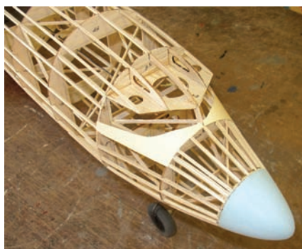
Rounded formers and external stringers give the DC-6 its final shape.
